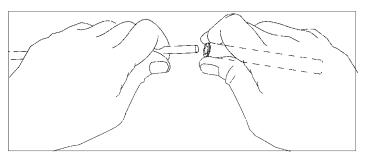
**lightly** clamped up against opposite button insulator will help maintain center reference (if you push the first retainer too far, remove element from boom, push retainer completely off the element, and start over). Install another retainer to the opposite side of the element. Continue installing retainers until all elements are secured.
