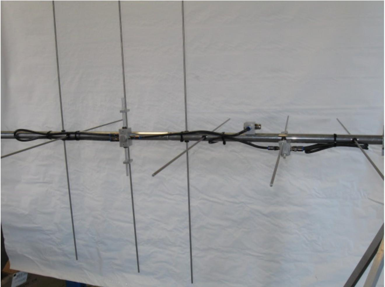
11. Use good quality coax and "N" connector for your feedline (see Installation Tips). Secure feed coax near connector on Junction Block, to provide stress relief. Allow about 60" of coax to hang in a loop between the rear end of the boom and the reattachment point (at least 12" beyond element tips) on the mast or crossboom.
