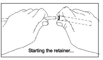
button. Locking pliers, *lightly* clamped up against opposite button insulator will help maintain center reference (if you push the first retainer too far, remove element from boom, push retainer completely off the element, and start over). Install another retainer to the opposite side of the element. Continue installing retainers until all elements are secured.
