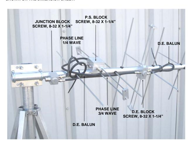
9. Viewed from the rear of the boom (rearmost Reflector HORIZONTAL), the VERTICAL Driven Element Block mounts to the RIGHT hand side of the boom with the two Balun connectors oriented to the FRONT. Secure with 8-32 x 1-1/4" screw. Install the Shorting Bars as in step #7.
