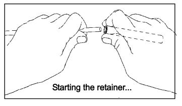
and continue until retainer butts on insulator button. Locking pliers, *lightly* clamped up against opposite button insulator will help maintain center reference (if you push the first retainer too far, remove element from boom, push retainer completely off the element, and start over). Install another retainer to the opposite side of the element. Continue installing retainers until all elements are secured.
