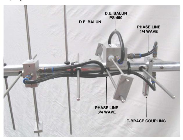
INSTALLATION OF THE *VERTICAL* DRIVEN ELEMENT BLOCK DETERMINES THE CIRCULARITY OF THIS ANTENNA. THE ORIENTATION OF THE BLOCK FOR RHC - RIGHT HAND CIRCULARITY, IS SHOWN ON THE DIMENSION SHEET.
