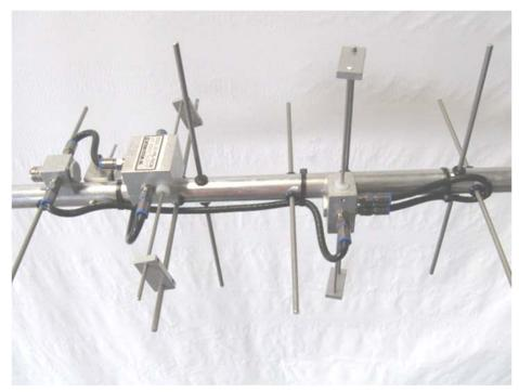
10. Use good quality coax and "N" connector for your feedline (see Installation Tips). Secure feed coax near connector on Junction Block, to provide stress relief. Allow about 60" of coax to hang in a loop between the rear end of the boom and the reattachment point (at least 12" beyond element tips) on the mast or crossboom. *Do not route feedline to boom to mast plate as exiting antenna here will adversely affect circular field.*
