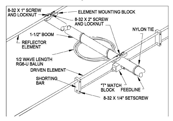
to the underside of the boom. Orient the match block with the "N" feed connector pointed to the front. Mount the remaining DIRECTOR ELEMENTS. Carefully note lengths on Dimension Sheet:.
