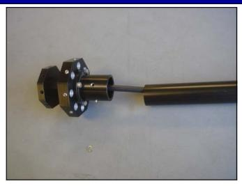
Zinc paste has been provided to lubricate during assembly and reduce long term corrosion. A small amount should be used on every screw thread, and on each metal to metal joint.
