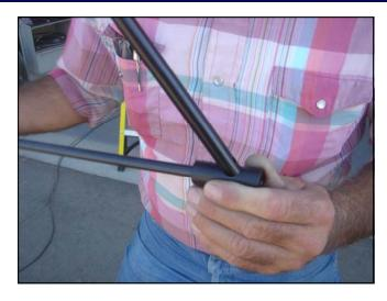
4. Raise the assembly and begin installing the support spokes as shown. Install 1-/4-20 set screws in the spoke hub and in the ends of the spokes as shown. Insert the spokes into the hub and tighten the inner set screws.
