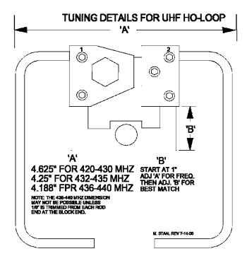
The 432 HO loop comes partially assembled from the factory only slight adjustment of loop size and/ or shorting bar may be necessary .
