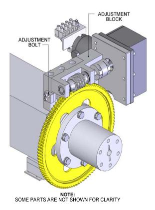
Excessive backlash may develop after using system for some time. We have incorporated a built in backlash adjustment block to keep backlash at a minimum.
