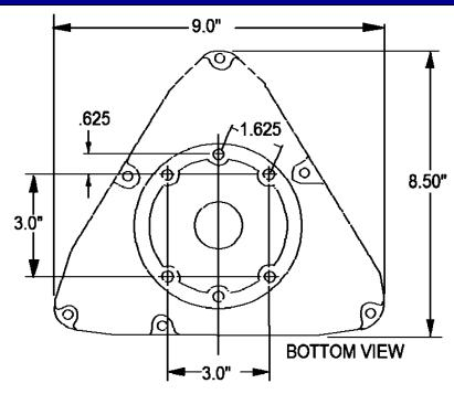
NOTE: FOR MAST DIAMETERS OVER 2-1/2" CONTACT M2 FOR LONGER BOLTS 3/8-24 X 4"
