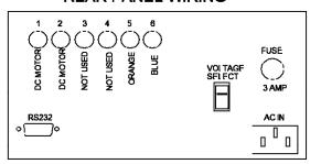
UNUSED WIRES IN YOUR CABLE CAN BE PARALLELED WITH THE MOTOR LEADS FOR MORE MOTOR TORQUE. WHEN USING BELDEN 9405 OR EQUIVALENT. TIE THE GREEN, BROWN, AND BLACK (MOTOR) LEADS TOGETHER. TIE THE YELLOW. RED AND WHITE (MOTOR) LEADS TOGETHER.
