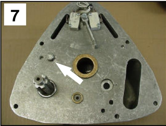
Once the new reed switch is installed, put the torque plate back onto the bottom casting and tighten the 1/4-20 bolt. Be very careful of the wires under the torque plate, as you can crimp them in between the two surfaces and cause more problems later.
