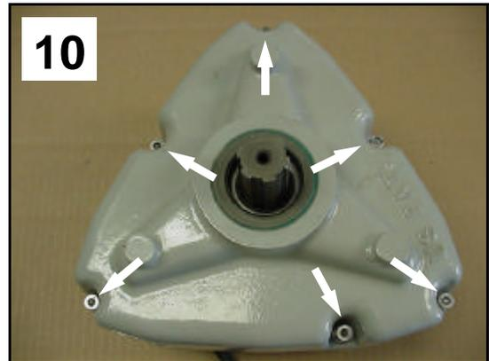
Install the (6) 1/4-20 internal hex bolts into the top casting and tighten.
