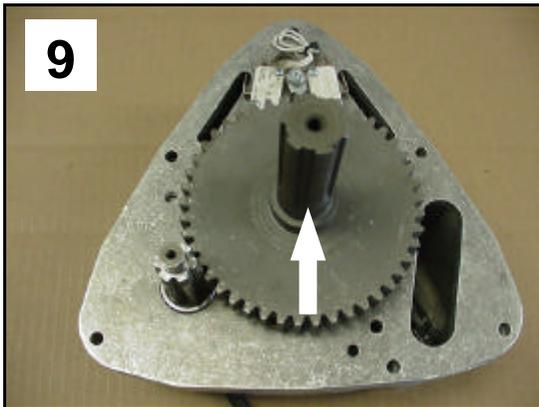
Once you are confident that the reed switch is working properly, reinstall the Gear #1 and shaft back into the torque plate. The position of the Gear #1 is not critical at this point. Once the unit is completely assembled, you can refer to your manual for calibration.
