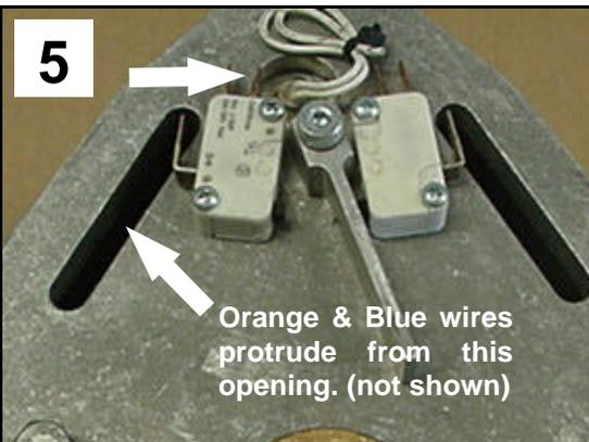
The reed switch is located at the top of the limit switches. The switch is tied in with the Orange & Blue wires coming from the bottom casting (not shown in picture)
