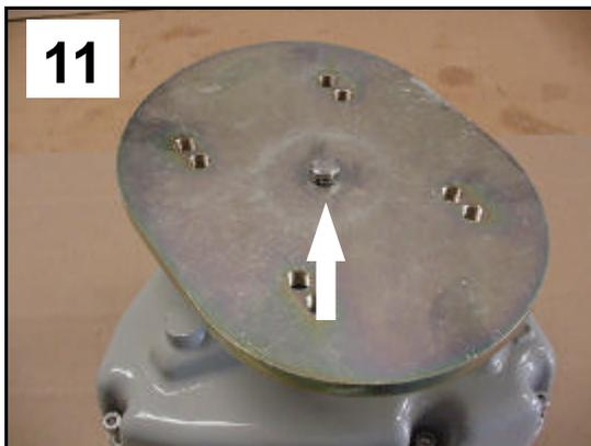
Intall the 1/4-20 Bolt with a 7/16 open end wrench or a socket. Make sure that this bolt is nice and tight.
