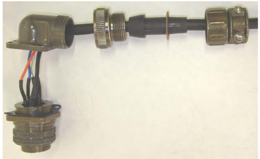
7 PIN RIGHT ANGLE FEMALE CONNECTOR WIRING
