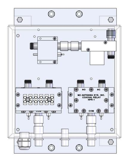
Terminal assignments are very important, so take your time when doing the wiring. Damage can be caused to the Preamp and Power Relays if connections are made incorrectly. \*Wiring detail is for a MAP65 System.
