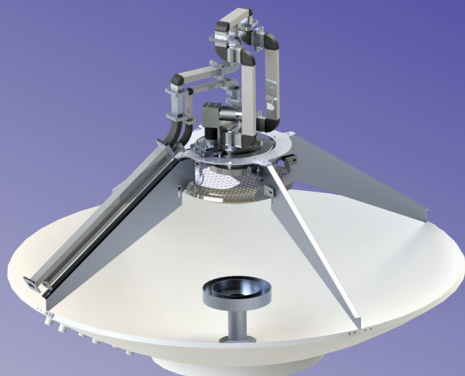
Tri-Band S-Band / C-Band & X-Band dish feed using Frequency Selective Sub Reflector
