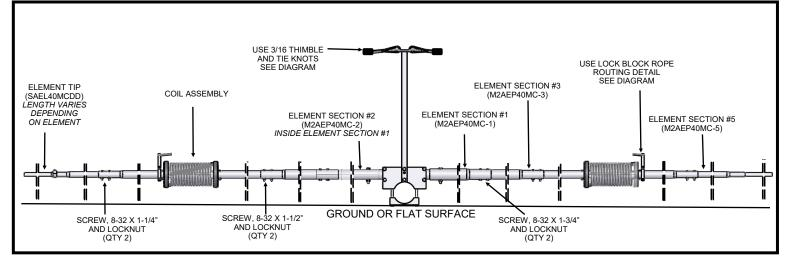
**NOTE:** For the final assembly on all the elements, it is best to perform the next steps on the ground or long flat surface. This will aid during final adjustment of the ELEMENT OVER HEAD SUPPORT. The ELEMENT HALVES are symmetrical on both sides. Do each of the following steps on both sides of the ELEMENT.
