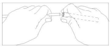
**lightly** clamped up against opposite button insulator will help maintain center reference (if you push the first retainer too far, remove element from boom, push retainer completely off the element, and start over). Install another retainer to the opposite side of the element. Continue installing retainers until all elements are secured.
