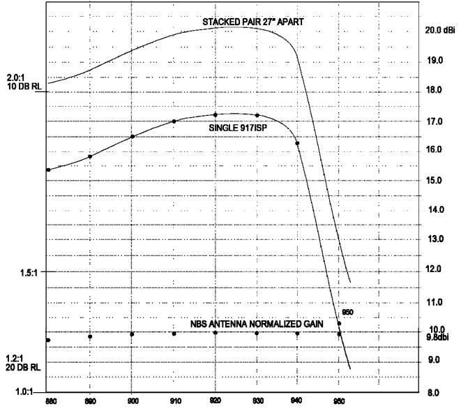
These are the actual gain curves taken using a pair of identical NBS refernce standard antenness which were built to to NBS dimensions for use at 840-950 MHz.
