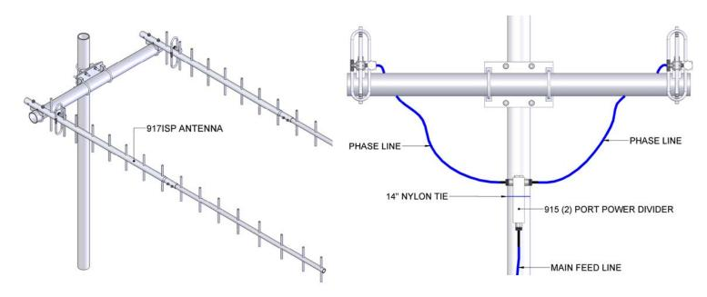
Attach the other pre-assembled 917-ISP to the right side of the 30" crossboom. Now attach the other phasing cable to the antenna and route to the right of the crossboom and underneath. Note— Both dipoles must be on the same side of the boom for proper phasing. **DO NOT MIRROR.**
