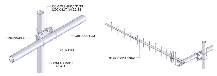
Attach the mounting plate to your vertical mast using U-bolts, Uni-Cradles, nuts and lock washers. Attach the 30" crossboom to the mounting plate using the same hardware. Make sure to cente the boom. The total distance between the two antennas will be 27".
