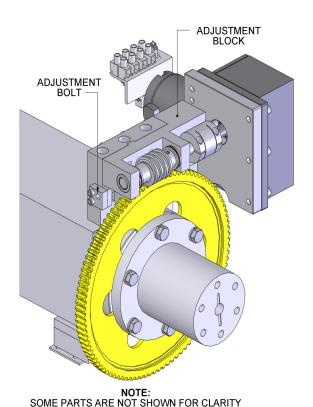
Excessive backlash may develop after using system for some time. We have incorporated a built in backlash adjustment block to keep backlash at a minimum.
