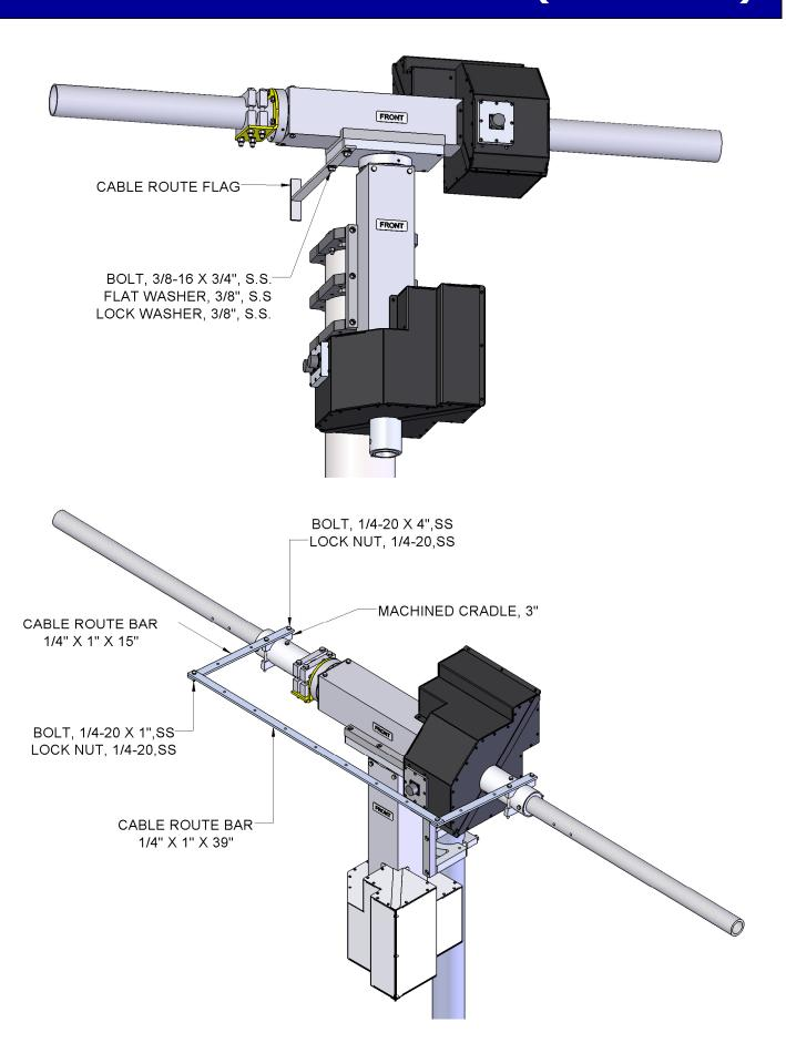
**Note:** The starting point for all cables that move with AZ or EL rotation. The AZ is at full counter clockwise and EL at 0 degrees.
