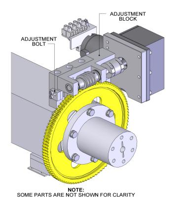
Excessive backlash may develop after using system for some time. We have incorporated a built in backlash adjustment block to keep backlash at a minimum.
