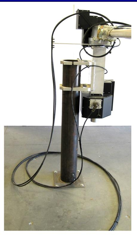
Note: The axis control cables and the RF cables are not tied together as the RF cables will rotate as the system articulates.
