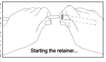
Locking pliers, lightly clamped up against opposite button insulator will help maintain center reference (if you push the first retainer too far, remove element from boom, push retainer completely off the element and start over). Install another retainer to the opposite side of the element. Continue installing retainers until all elements are secured.
