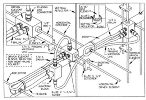
lightly clamped up against opposite side of the element. Continue installing retainers until all elements are secured.
