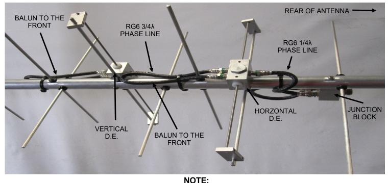
INSTALLATION OF THE D.E. BLOCKS DETERMINES THE CIRCULARITY OF THIS ANTENNA. THE ORIENTATION OF THE BLOCKS FOR RHC - RIGHT HAND CIRCULARITY, IS SHOWN ABOVE, BELOW & ON THE DIMENSION SHEET.
