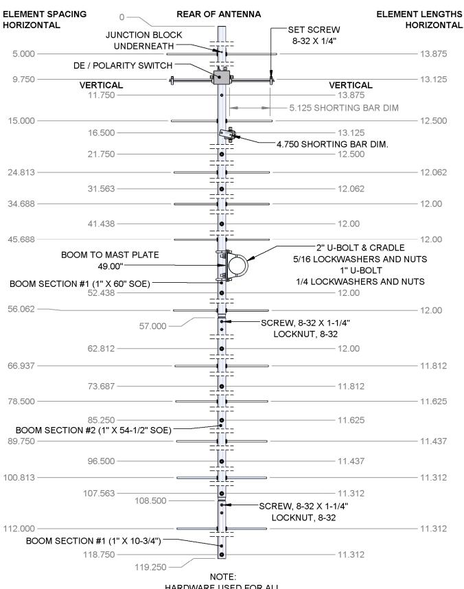
HARDWARE USED FOR ALL D.E. / P.S. BLOCKS SCREW, 8-32 X 1-1/4, SS LOCKNUT, 8-32, SS
