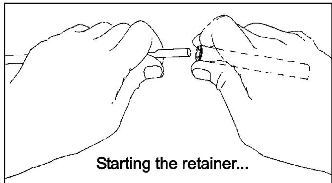
3. Install the 3/16" rod DRIVEN ELEMENT as you did the reflector. Then continue with the installation of the DIRECTORS. **Note: the Director Elements do not consistently diminish in length from rear to front, so pay close attention to length and position.**
