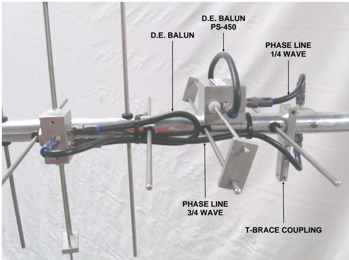
**INSTALLATION OF THE VERTICAL DRIVEN ELEMENT BLOCK DETERMINES THE CIRCULARITY OF THIS ANTENNA. THE ORIENTATION OF THE BLOCK FOR RHC - RIGHT HAND CIRCULARITY, IS SHOWN ON THE DIMENSION SHEET.**
