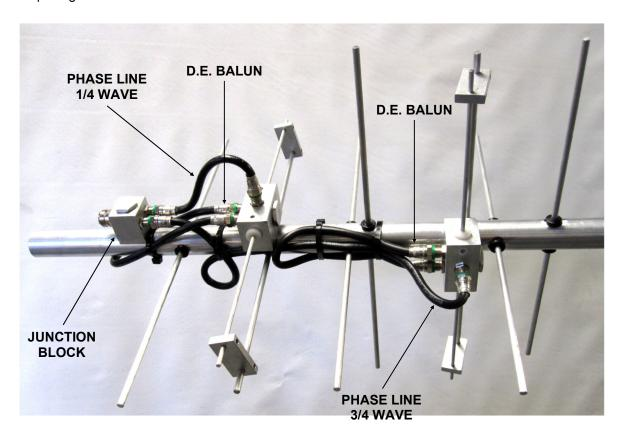
NOTE: USE 8-32 X 1-1/4" SCREW FOR D.E. BLOCKS AND JUNCTION BLOCK.
