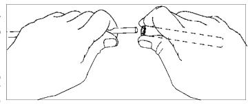
element end and continue until retainer butts on insulator button. Locking pliers, *lightly* clamped up against opposite button insulator will help maintain center reference (if you push the first retainer too far, remove element from boom, push retainer completely off the element, and start over). Install another retainer to the opposite side of the element. Continue installing retainers until all elements are secured.
