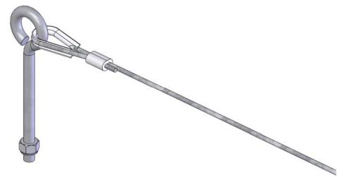
Wire rope assembly half is pre-assembled at factory as shown above. Complete the other end of the assembly using the supplied wire nuts, cable eye and turnbuckle as shown below. In some
