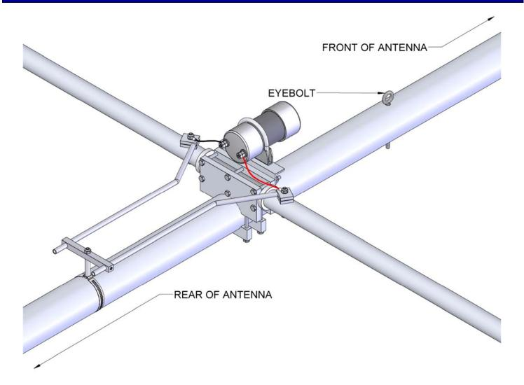
**NOTE:** HAIRPIN HAS BEEN ROUTED TO THE REAR OF ANTENNA TO AVOID INTERFEARENCE WITH OVERHEAD SUPPORT EYEBOLT.
