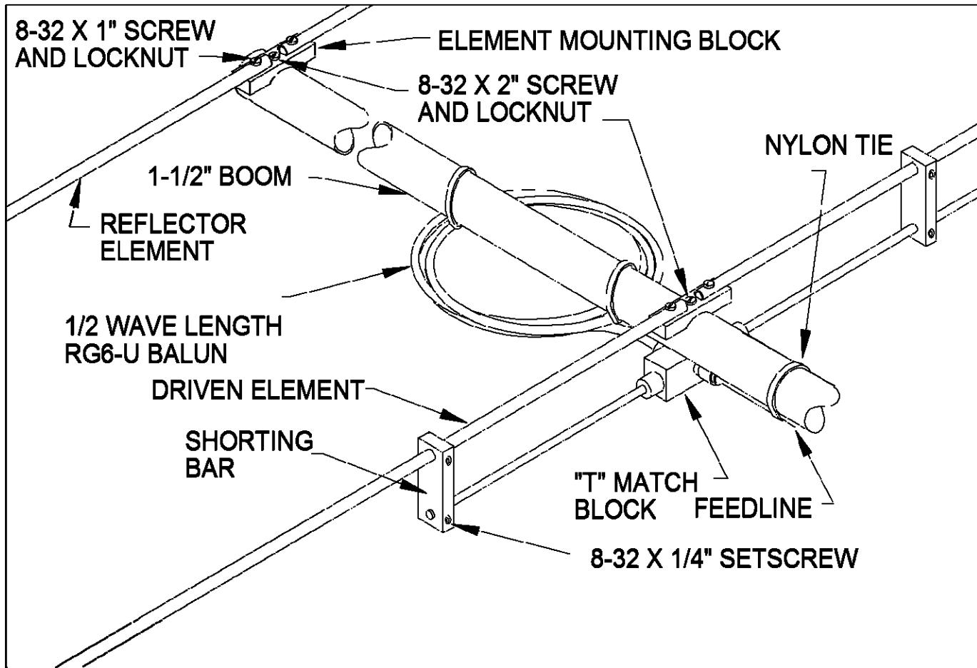
to the underside of the boom. Orient the match block with the "N" feed connector pointed to the front. Mount the remaining DIRECTOR ELEMENTS. Carefully note lengths on Dimension Sheet:.
