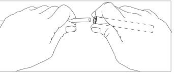
button insulator will help maintain center reference (if you push the first retainer too far, remove element from boom, push retainer completely off the element, and start over). Install another retainer to the opposite side of the element. Continue installing retainers until all elements are secured.
