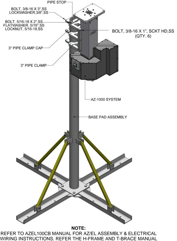
WIRING INSTRUCTIONS. REFER THE H-FRAME AND T-BRACE MANUAL FOR H-FRAME ASSEMBLY INSTRUCTIONS. EACH ANTENNA WILL HAVE IT'S OWN MANUAL WITH ASSEMBLY INSTRUCTIONS.
