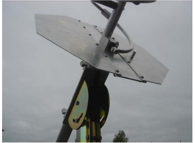
PHOTOS OF RANGE TEST SETUP AND CLOSE UPS OF THE FEED SYSTEM AND THE MANUAL TILT MECHANISM.
