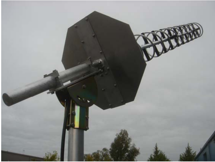
PHOTOS OF RANGE TEST SETUP AND CLOSE UPS OF THE FEED SYSTEM AND THE MANUAL TILT MECHANISM.
