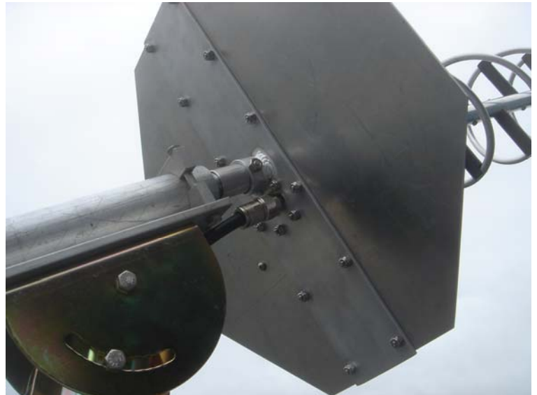
PHOTOS OF RANGE TEST SETUP AND CLOSE UPS OF THE FEED SYSTEM AND THE MANUAL TILT MECHANISM.
