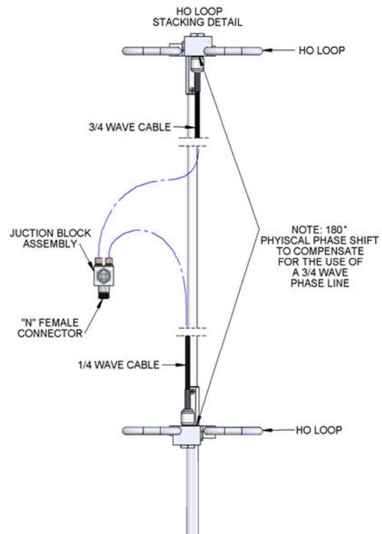
Mount both antennas with no phasing cables installed. Make sure the feed connectors are facing each other and the larger feed blocks are on the opposite side on each antenna. (2M and 222 only). Creating a 180° phase shift.
