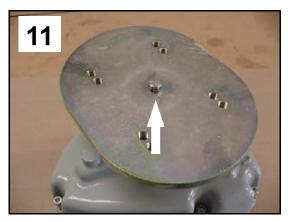
Intall the 1/4-20 Bolt with a 7/16 open end wrench or a socket. Make sure that this bolt is nice and tight.
