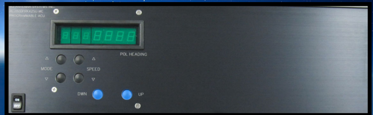
THE FGRC2800PRKX1SU SINGLE AXIS POLARITY CONTROLLER
