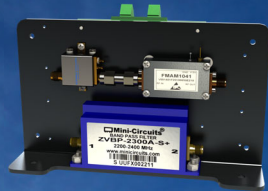
Low Noise Amplifier and Filter On custom M2 replaceable blade
