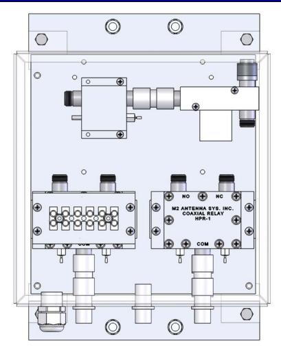
Terminal assignments are very important, so take your time when doing the wiring. Verify voltages on **M2 EME S2 Sequencer** before connecting to the housing. Damage can be caused to the preamp and power relays if connections are made incorrectly. \*Wiring detail is for a MAP65 System.
