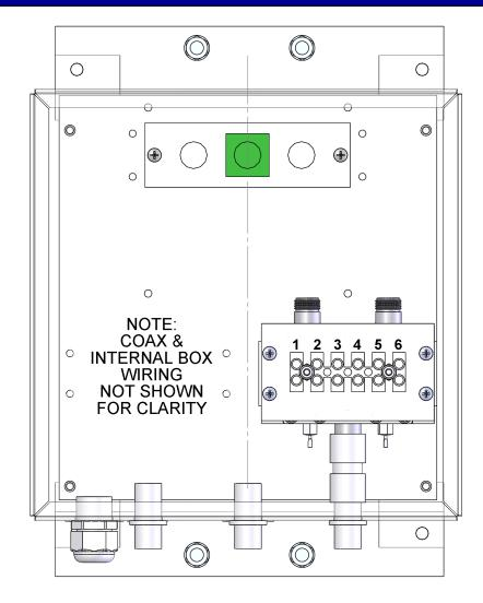
Terminal assignments are very important, so take your time when doing the wiring. Damage can be caused to the Preamp and Power Relays if connections are made incorrectly. \*Wiring detail is for a Single Polarity System.
