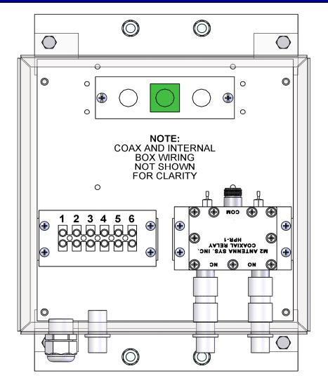
Terminal assignments are very important, so take your time when doing the wiring. Damage can be caused to the Preamp and Power Relays if connections are made incorrectly.
